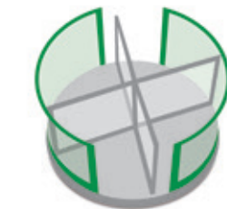
IDC/KBB drum wall load-bearing
