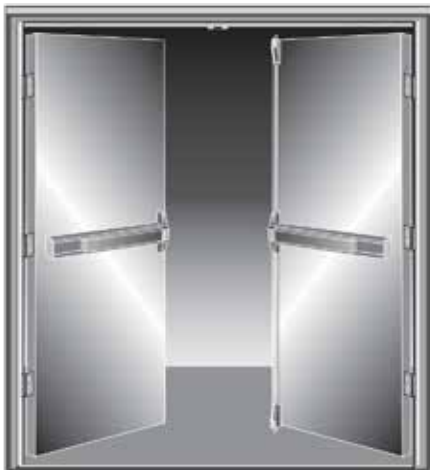
One Rim Device and one Surface Vertical Rod Device combination - same direction
