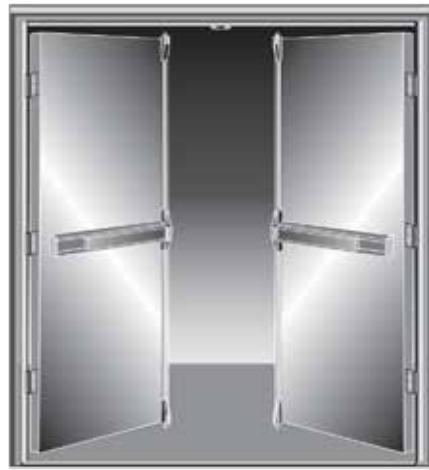
Two Surface Vertical Rod Devices - same direction (do not use with overlapping astragal)
